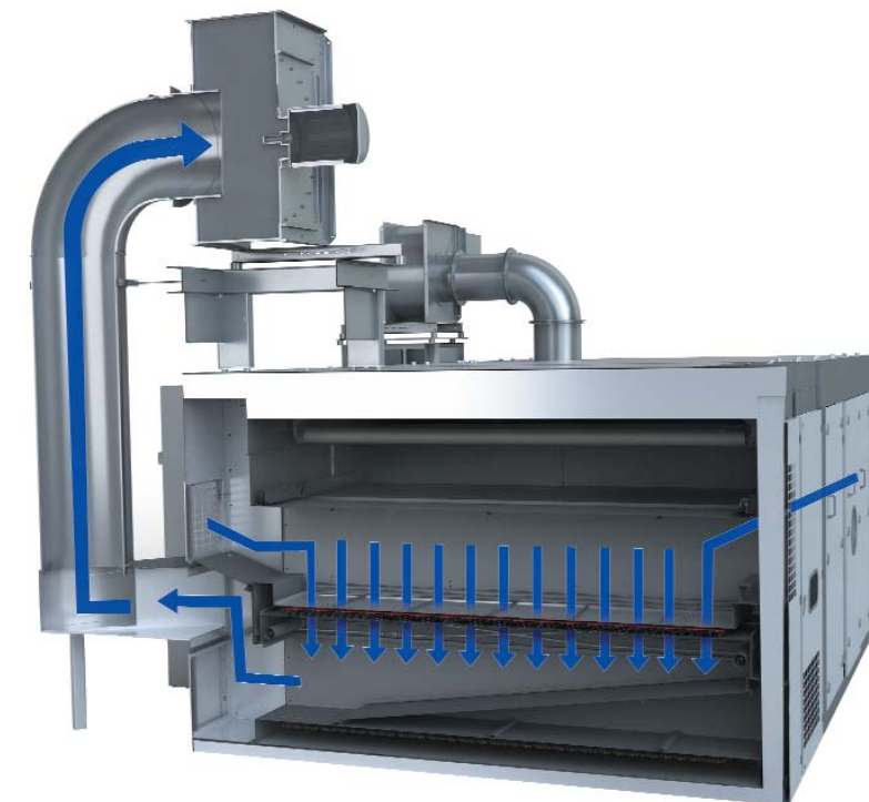
Air flow across the width cooling zone
