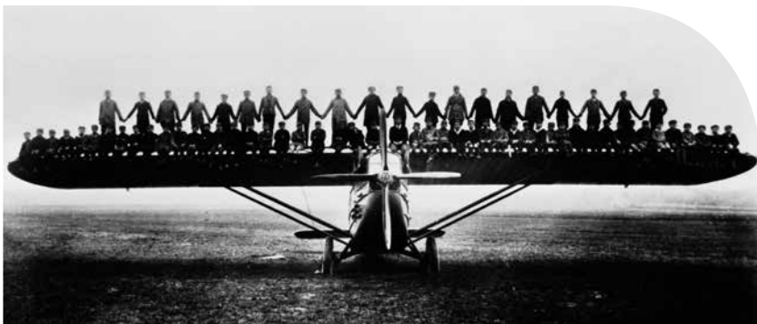
Endurance test and group photo on a Dornier Komet II in all-metal construction, around 1922.
