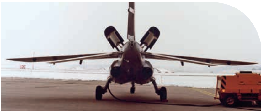
Dornier/Dassault Alpha Jet with extended CFRP speedbrakes, around 1973.
