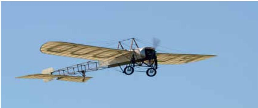
Aircraft Blériot XI with textile fiber covered wood construction, around 1909.
