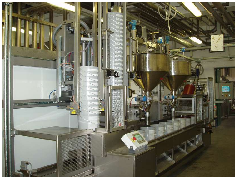
Automatic pail denester type V420, incorporated in a De Vree twin volume filler.
